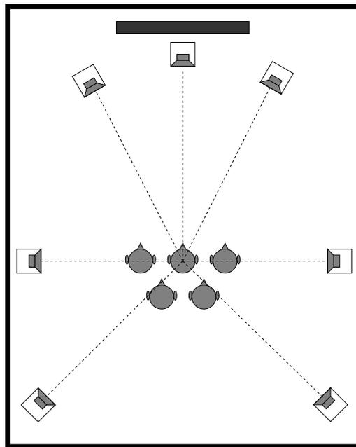
**Figure 1:** Typical loudspeaker positions in a 7.1-channel surround sound system. The prime listening position is the position where the lines drawn from each loudspeaker converge. Copyright 2019 from *Optimal Audio and Video Reproduction at Home* by Vincent Verdult (figure 4.1). Reproduced by permission of Taylor and Francis Group, LLC, a division of Informa plc.
