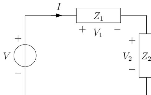
**Figure 9:** In this series connection of two impedances  $Z_1$  and  $Z_2$  the sum of the voltages  $V_1$  and  $V_2$  equals the supply voltage  $V$ .
