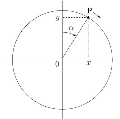
**Figure 3:** The position of the point  $P$  on the circle can be described by the angle  $\alpha$ .
