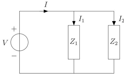
**Figure 8:** In this parallel connection of two impedances  $Z_1$  and  $Z_2$  the sum of the currents  $I_1$  and  $I_2$  equals the supply current  $I$ .
